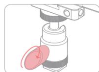
② Adjust the angle of the ball head adapter as required and secure using the adjuster.
