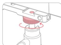
① Turn the 1/4 screw located on the adapter into the screw hole found on the LED light holder and tighten using the locking ring.
