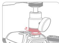
③ Slide the hot shoe base piece of the adapter into the camera's hot shoe and tighten the base locking ring.
