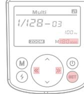
2: Press the "SET" button until a flashing "----" is displayed on the screen allowing you to fine-tune the settings.
