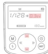
3: Diagram: 0EV → +0.3EV → +0.7EV 0EV → -0.3EV → -0.7EV. Press the "^" or "V" button to fine-tune the power value.
