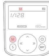
1: Press the "M" mode button until "M" is displayed at the top of the screen.
