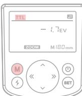
1: Press the "M" mode button until a "TTL" is displayed at the top of the screen.
