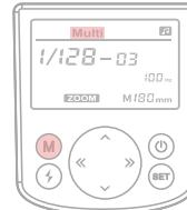
1: Press the "M" mode button until "Multi" is displayed at the top of the screen.
