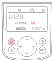
1: Press the "M" mode button until "S2" is displayed on the screen.
