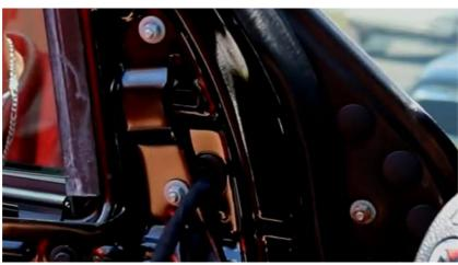
Align the tab on mirror base with the slot on door panel. Attach new mirror and finger tight three 10mm hex nuts.
