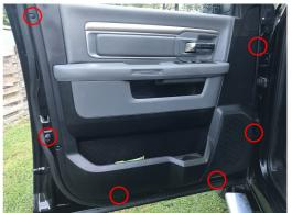
Lift and release inner door panel away from front door. Disconnect door lock harness.
