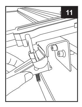
\*Line the bracket up with the tri-fold cover clamp location once they are lined up. Secure bracket to the vehicle bed rail.
