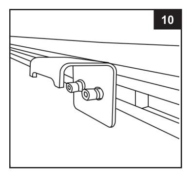
\*Attach the clamp bracket to the plate with the included Allen head bolts.
