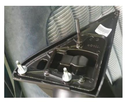
2.2. Tighten the lower 2 nuts and place the metal reinforce bracket.
