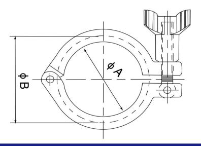
Material: Tri-Clamp Coupling, Wingnuts and Eye-Bolt Screw fromSS 304
