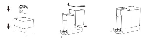
3. Fill the feed water tank and discard the first two tanks of filtered water to fully flush the filter cartridge before starting to use.
