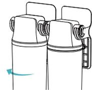
› Step 2: Using the wrench to unscrew the housing body
