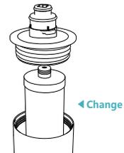
› Step 4: Flush the new cartridge for 15 minutes before starting to use
