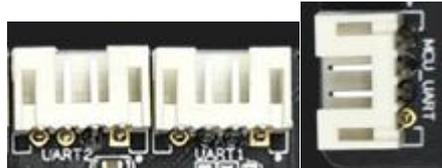
The board leads out two groups of common UART serial ports, which can support common UART serial port devices on the market.
