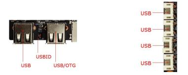
The motherboard has 2 USB standard interfaces and 4 USB pins
