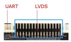
General LVDS interface definition, support single/dual, 6/8/10 bit 1080P LVDS screen. The screen voltage can be selected through the bridle-wire cap, and can choose to support 3.3V/5V/12V screen power supply.
