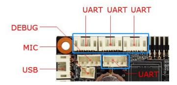
The motherboard leads to two sets of common UART serial ports, which can support common UART serial devices on the market.
