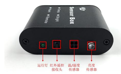
**Running light:** flicker—work; not bright—Not working (check the cable if it is reversed connected.); Press the remote control and it will flash.
