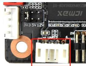
The motherboard leads to one set of common UART serial ports, which can support common UART serial devices on the market.
