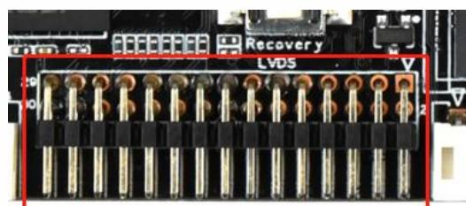
General LVDS interface definition, support single/dual, 6/8/10 bit 1080P LVDS screen. The screen voltage can be selected through the bridle-wire cap, and can choose to support 3.3V/5V/12V screen
