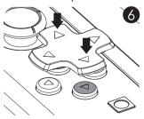
Attach the D-pad to the buttons
