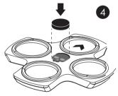
Attach the BLACK PAD to the back of D-pad as a pivot
