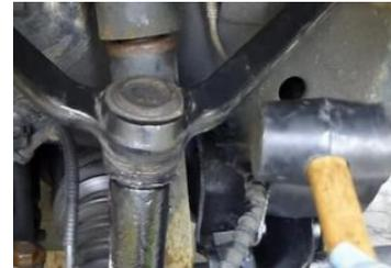
7. Loosen the control arm nuts on both sides.
