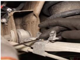
4. Mark the control arm position. Before loosening any of nuts, you need to mark off the control arm's position.
