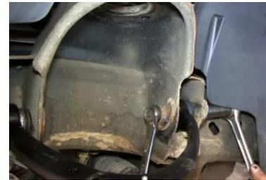
8. Remove old Control arms and then install new control arms. Adjust the control arm alignment to the marked area. Mount the control arm ball joint to the hub assembly.
