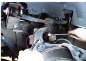
6. Using a hammer, hit the side of the knuckle attached to the upper control arm's ball joint. Continue hitting the knuckle until the ball joint has been freed.
