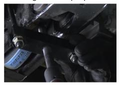
7. Using a 21mm socket rotate the tool bowl upward against the factory key just enough to unload the key from the block.
