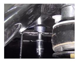
19. Install the remaining center bolt and spacer in the same way.
