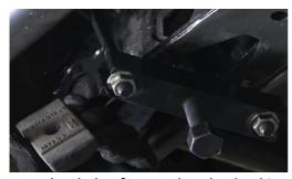
9. Unload the factory key by backing off the tool bolt until the key is free of tension.
