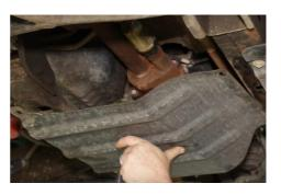
18. Put one of the supplied spacers on top of the pan and screw one of the supplied bolts as shown.
