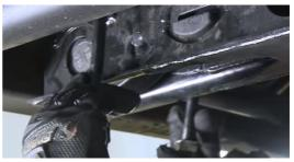
16. The precise height adjustments will be made during the alignment. For now, you need to tighten up the adjuster bolt just enough so it sits nearly flush with the bottom of the cross-member.
