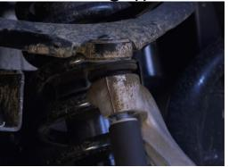
8) Disconnect the strut from the lower control arm.
