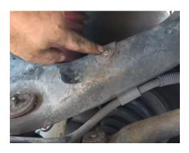
3. Mark the control arm position. Before loosening any of nuts, you need to mark off the control arm's position.
