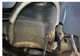
8. Remove old Control arms and then install new control arms. Adjust the control arm alignment to the marked area. Mount the control arm ball joint to the hub assembly.
