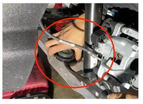
7.Remove the trailing arm bolts on the frame.
