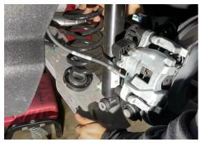
6.Remove the rubber spring seat with a flathead screwdriver.
