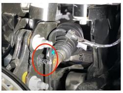
7.Remove the brake line bracket with an 8mm wrench. Do not disconnect any hydraulic brake lines. Retain factory hardware.
