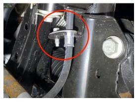
8.Remove the 21mm lower strut nuts on the knuckle. Use a hammer to remove the bolts from the knuckle. Retain factory hardware.
