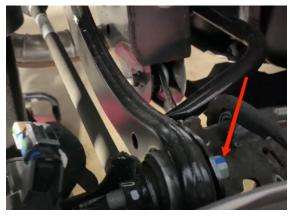
5.Push down on the control arm to free the spring from the control arm, a flathead screwdriver may be needed to remove the lower spring pad from its location.
