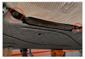
3.Remove the lower shock bolt using a 15mm socket / wrench.
