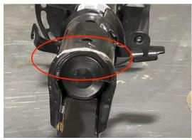
11.Install the front strut spacer with the factory bolts. Spacers are identical and strut bolt pattern is asymmetric, allowing only one installation orientation. Tighten bolts evenly until spacer is flush to strut.
