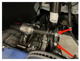
9.Remove upper strut bolts using a 13mm socket and remove strut from vehicle.
