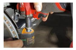
(Strike the side of the steer arm to remove the tie rod from the knuckle.)
