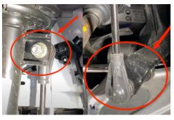
6.Use a trim removal tool to remove the ABS wire clip from the knuckle.
