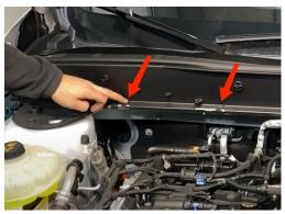
3.Lift up the cowl and remove the bolts for the upper strut cover using a 10mm wrench. Remove upper strut cover.
