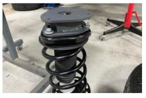
12.Install the strut and front strut spacer assembly into the vehicle using the supplied M8-1.25 x 25mm flange bolt.
