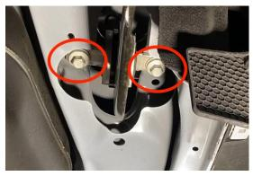
8.Install the trailing arm drop spacers between the mount and the body of the vehicle and secure with the supplied M14x2.0 bolts.
