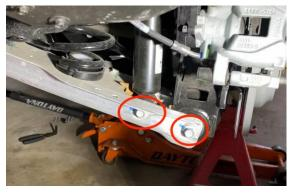
4.Loosen the control arm bolts but do not remove, to allow the trailing arm / hub and brake combo to droop more easily.
