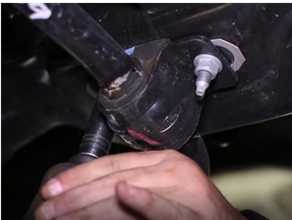
7) now the sway bar frame mounts can be removed and a sway bar can either be taken off the truck.
