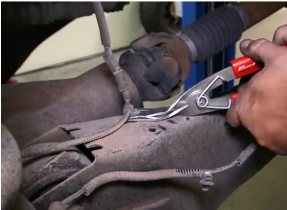
7) now the sway bar frame mounts can be removed and a sway bar can either be taken off the truck.
