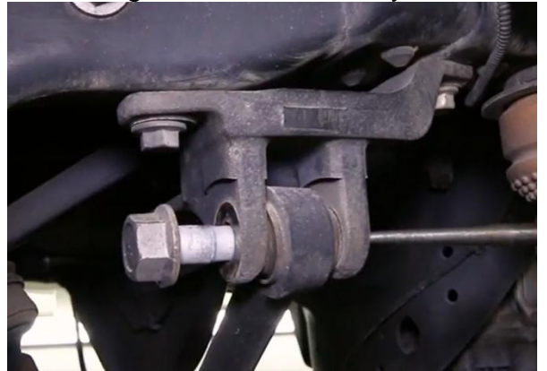
11) Disassemble the factory bump stops by pulling out the stop itself. Then unbolting the top plate from the track bar.
