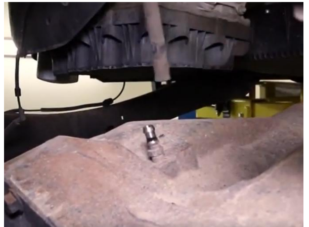
10) Remove the bolt that holds the track bar which can be unbolted from its bracket and swung down out of the way.
