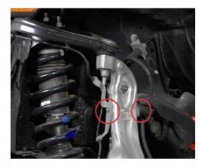
5. Using a pry tool or pliers remove brackets from control arm.
