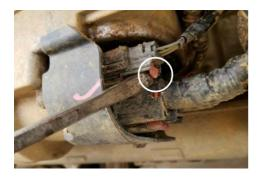
4. Remove the abs wire bracket from the front side of the knuckle with a 8mm socket. Remove the brake line bracket from the back side of the knuckle with a 10mm socket. Remove abs sensor from the top of the knuckle with a 8mm socket.
