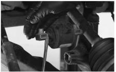
8. Place strut spacer under the lower strut mount and align holes. The "U" shaped portion of the spacer will wrap down around the backside of the control arm mount.
