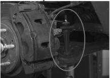
3. Using an 18mm wrench loosen the upper strut bolts. It is not necessary to remove nuts.
