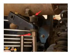
13. Install Rear Brackets by small bolts to Lower A-Arms with hardware shown.
