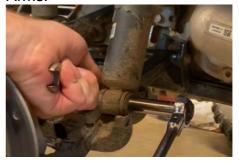
Remove top bolts from Torsion Bar.
