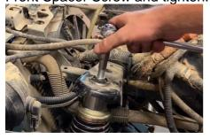
7. Reinstall Top Washer and Lock Nut.
