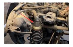
6. Push the Strut back and place Strut Assembly in Frame using new Front Spacer Screw and tighten.
