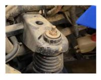
3. Remove Lock Nut, Washer, and Plastic Bearing from top of Strut Assembly.
