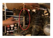
12. Install Hex Spacers on top of exsisting Hex Bar . Install new longer bolt through assembly. Rubber Bushings must go back to original
