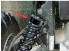
We suggest that re-tightening all bolts and nuts on the lift kits after 100-200 miles of driving.
