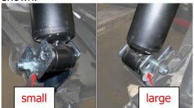
NOTE: The Large Brackets install to inside of Shock Bracket. The Small Brackets mounts to outside of Shock Bracket.
