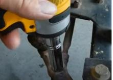
4. Remove three bolts from rack and pinion. Retain Hardware.
