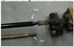
11. Install new steering riser on spindle using supplied hardware. Install rack ball joint on steering riser using retained hardware.
