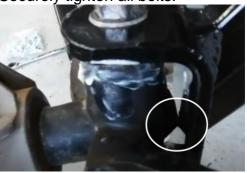
Note: Some spindle had a casting that needed to be ground down. For the spindle to turn full motion
