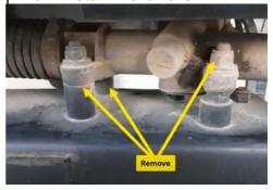
5. Remove the lower washer, bushing, and nut from shock. Push shock up and out of the way. Retain Hardware. Remove five bolts from factory axle. Retain shock plates and hardware.
