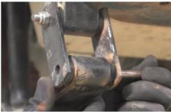
4.Install Rear Riser on top of the axle using supplied hardware. Note: the angle of Rear Riser should be the same as leaf spring.
