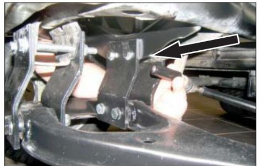
Spacer Placement in Riser
