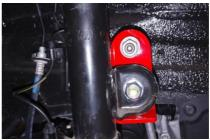
12. Install the wheels and lower the vehicle to the ground. Torque the lug nuts to the wheel manufacturer's specs. Torque the upper strut hardware to 30 ft-lbs. (Stept 7)
