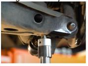
5.Remove the fastener which connecting the stabilizer bar with the control arm.
