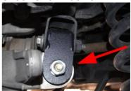
Repeat steps 13-20 on other side. Reinstall both sway bar links. Check all hardware is mounted at correct torque settings. Recheck all work, and reinstall wheels. Re-tighten Lower Control Arm mounting bolts. Test drive, then have a trained technician perform an alignment.
