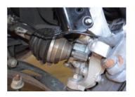
10.Install sway bar extension bracket with provided hardware. Tighten the sway bar end link to the bracket.
