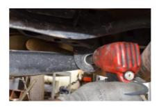
15.Support the LCA with a floor jack and remove the mounting bolt at the steering knuckle. Carefully lower
