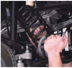
6. Install the front coil spacers and then put the isolator back on.
