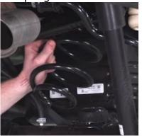
7. Install the washer nut in the strut recess.
