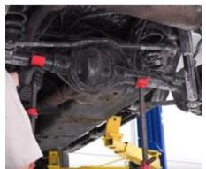
2. Remove the track bar and sway bar end links. Since there are new sway bar
