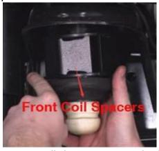
7. Reinstall the spring. Get the bump stop inside of the spring while installing. Be sure to rotate the spring until the pigtail hits the stop.
