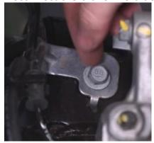
5. Disconnect the bottom of the shock.
