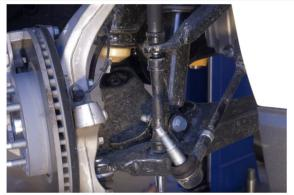
4) Remove the wheel speed sensor wiring bracket from the back of the steering knuckle.
