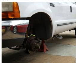
2) Remove the wheels to gain access to the hub and suspension components.
