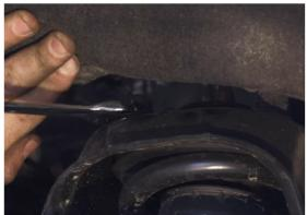
10) Install the strut spacer on to the top of the strut with the included hardware.
