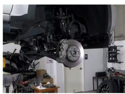
3) Disconnect sway bar links and upper ball joint nut.
