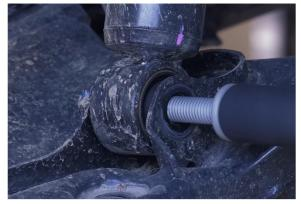
9) Remove the three upper strut mount nuts and remove the strut from the vehicle.
