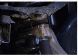
8) Disconnect the strut from the lower control arm.
