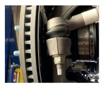
7.Remove the upper ball joint nut. Use an impact tool or ball-peen hammer and hit the steering knuckle until the upper control arm pops out.
