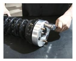
12.Run down nuts snug with an open end wrench. Torque to OEM specs.
