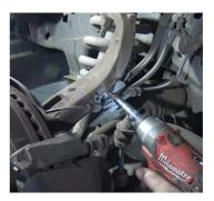
4. Remove the sway bar lower link pin bolt from the bottom of the control arm.
