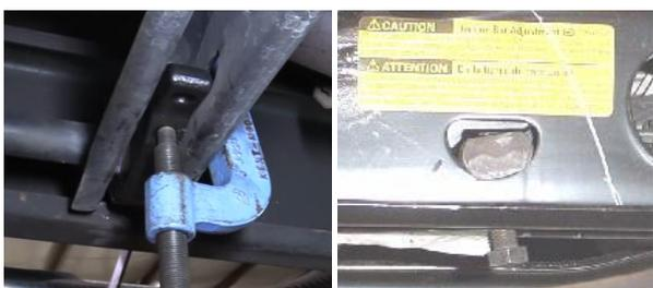
10. Torque all bolts in the installation torsion key to factory specs.
