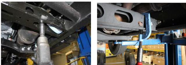
9. Install the new torsion key, and reinstall the bar pin and torsion bolt.
