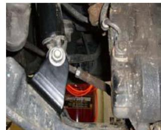
5. Install the lower shock and shock hardware to the new mount and torque to spec.
