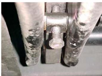
8. Working on the driver side, Remove the adjuster bolts from the torsion key.
