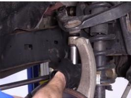
5. Hit the knuckle with hammer on the side to separate the ball joint from the knuckle, but don't let the knuckle to pull out so far that the
