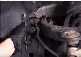
3. Mark the control arm position. Before loosening any of nuts, you need to mark off the control arm's position.
