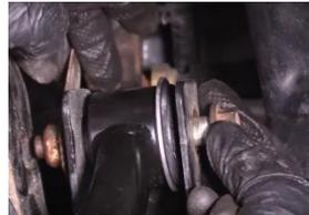
7. Remove old control arms and then install new control arms. First, reinstall the control arm nuts on both sides.
