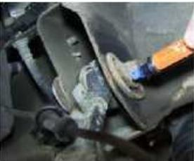
4. Loosen the upper ball joint nuts until there is a visible gap between the nut and spindle.
