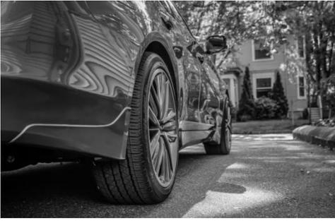
5. Check for proper tire clearance in the wheel well, making certain there is sufficient wheel and tire clearance for full steering (lock-to-lock). If there is no interference, vehicle may be lowered. Once vehicle is on the ground under full load, recheck for adequate tire and wheel clearance and unobstructed lock-to-lock steering. **NOTE : Re-torque all lug nuts on the spacer/adaptor after 25-50 miles of driving, then again after 1-2,000 miles.**
