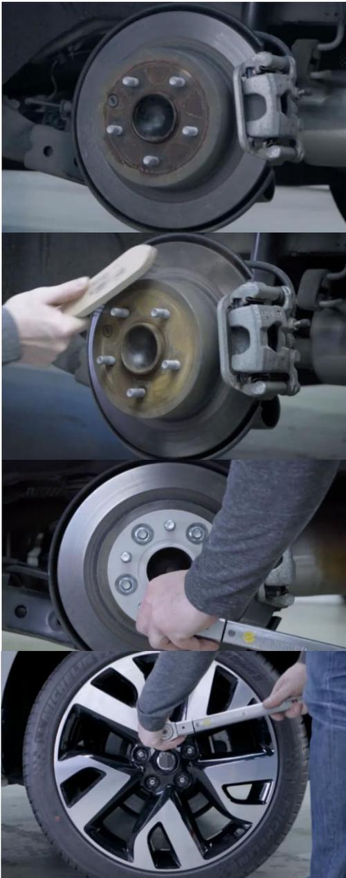
1. Following your vehicle owner's manual, properly raise the vehicle and support it using adequately load-rated jack stands. Never work on a raised vehicle that is supported with a factory emergency, floor or bottle jack. Remove wheels and inspect rotors for any damage or cracks. If any damage is identified, do not continue with this installation.
