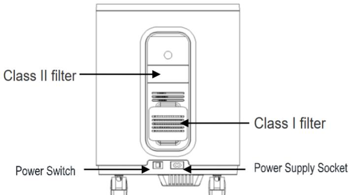
Figure 2: rear side view of the whole machine
