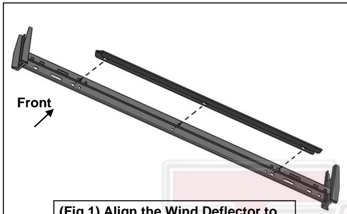
(Fig 1) Align the Wind Deflector to the front face of the Cross member
