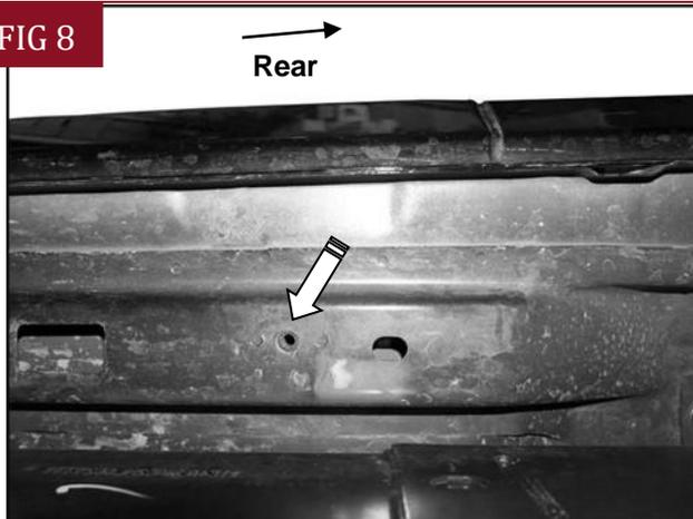
(Fig 8) Driver/Left rear mounting location (Model with threaded inset shown)
