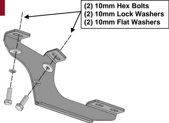
**(Fig 2) Attach (1) Front Mounting Bracket to the Passenger/Right front location**
