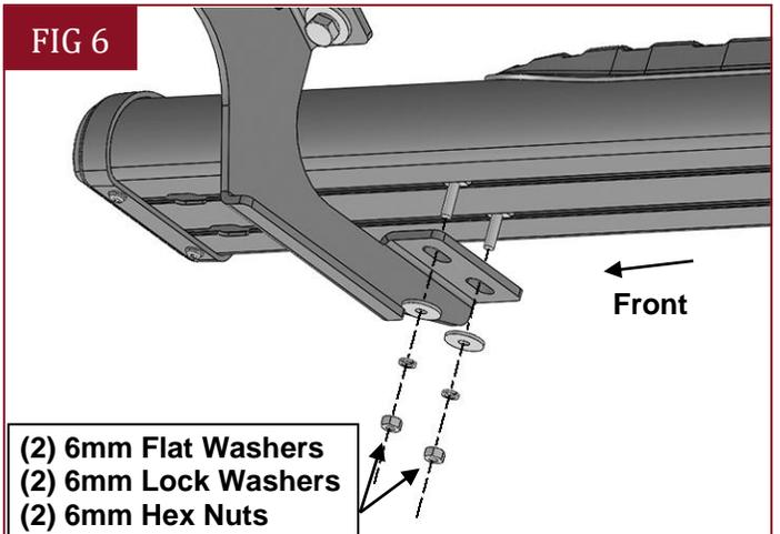
(Fig 6) Attach the Passenger/Right Side Step to the Mounting Brackets
