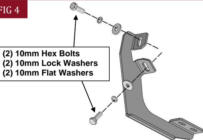
(Fig 4) Attach (1) Rear Mounting Bracket to the Passenger/Right rear location
