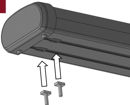
(Fig 5) Insert (4) 6mm T-Bolts into the channels in the bottom of the Side Step, (2 T-Bolts per channel)
