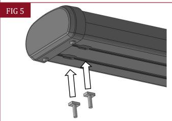
(Fig 5) Insert (4) 6mm T-Bolts into the channels in the bottom of the Side Step, (2 T-Bolts per channel)
