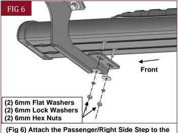
(Fig 6) Attach the Passenger/Right Side Step to the Mounting Brackets
