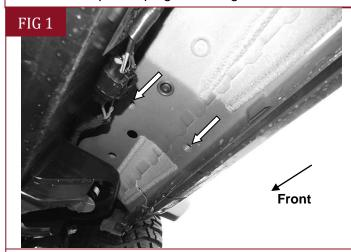
(Fig 1) Passenger/Right front mounting location
