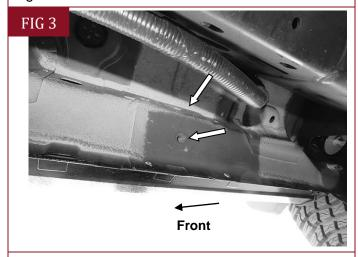
(Fig 3) Passenger/Right rear mounting location
