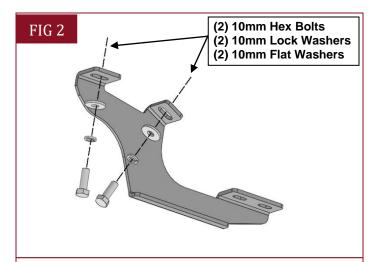
(Fig 2) Attach (1) Front Mounting Bracket to the Passenger/Right front location
