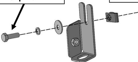
(Fig 15) Slide Upper Bracket over weld nut if equipped
