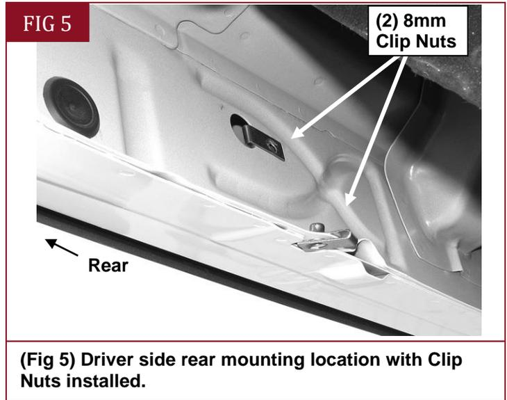
(Fig 5) Driver side rear mounting location with Clip Nuts installed.
