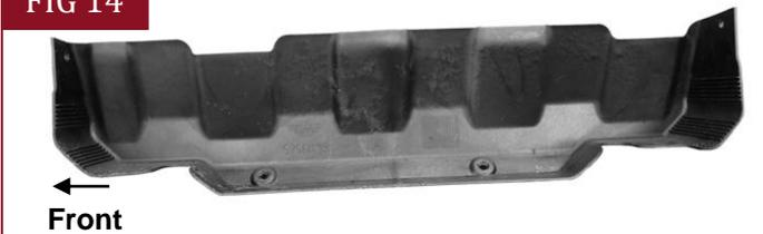
(Fig 14) 2017 Passenger side DEF cover removed
