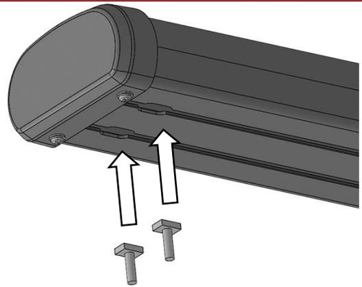
(Fig 9) Insert (4) 6mm T-Bolts into the channels in the bottom of the Side Step, (2 T-Bolts per channel)
