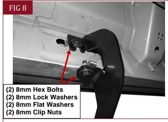
(Fig 8) Attach the Mounting Bracket to the <u>Clip</u> Nuts
