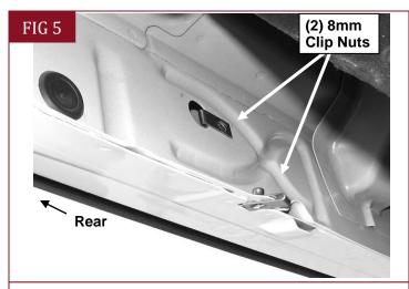
(Fig 5) Driver side rear mounting location with Clip Nuts installed.
