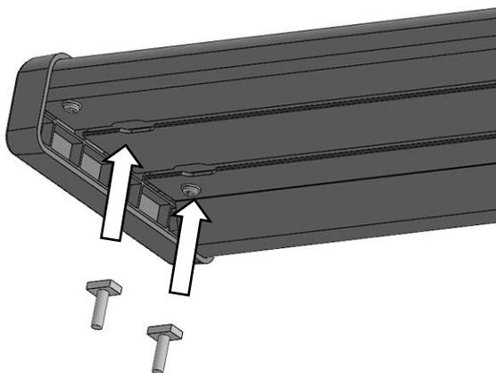
(Fig 5) Insert (6) 6mm T-Bolts into the channels in the bottom of the Running Board, (3 T-Bolts per channel)
