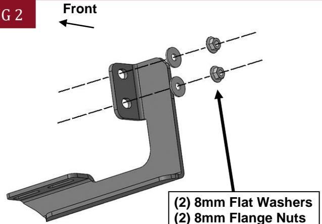
**(Fig 2) Attach (1) Mounting Bracket to the front location**
