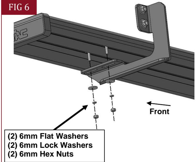
(Fig 6) Attach (1) Running Board to the Mounting Brackets
