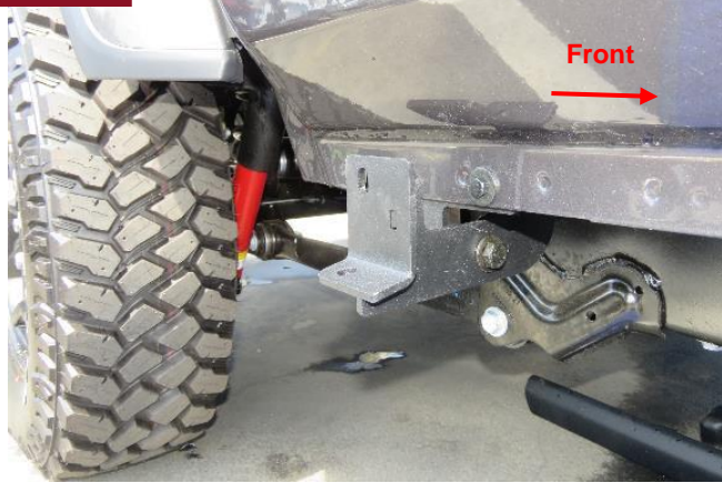
(Fig 12) Attach Passenger/Right Rear Bracket and Passenger/Right Rear Support Bracket to the rear location
