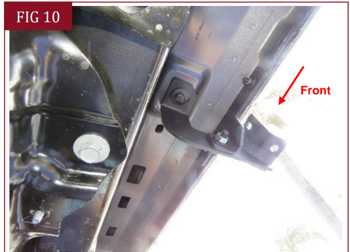
(Fig 10) Attach Passenger/Right Center Bracket and Passenger/Right Center Support Bracket to the center location
