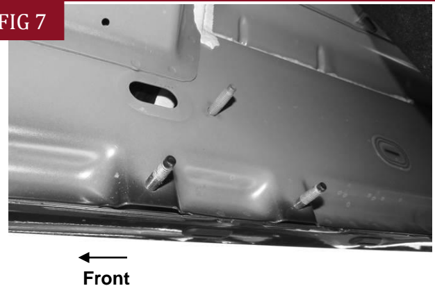
(Fig 7) Passenger/Right Center mounting location
