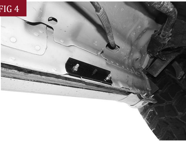
(Fig 4) Example of the Support Bracket (#1) attached to the threaded studs
