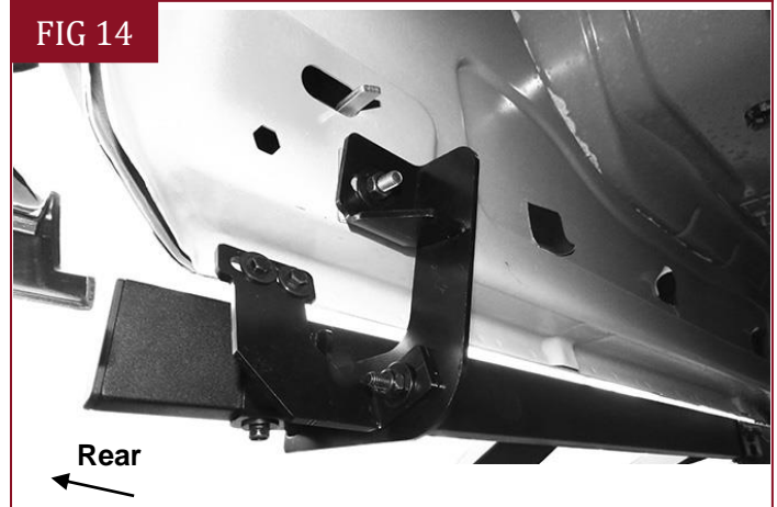
(Fig 14) Driver/left Side Step attached to Rear Brackets
