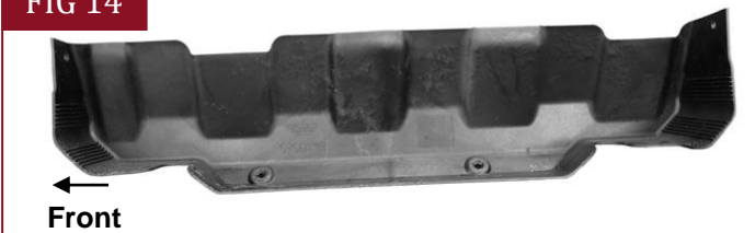
(Fig 14) 2017 Passenger side DEF cover removed
