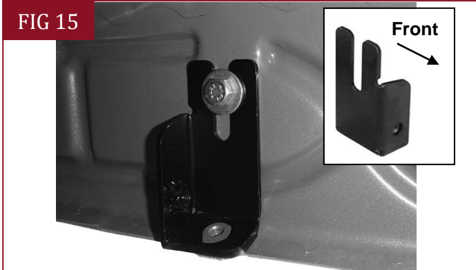
(Fig 15) Slide Upper Bracket over weld nut if equipped
