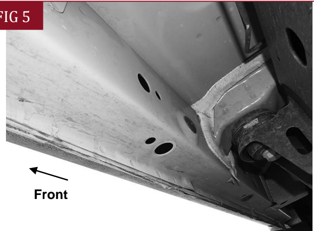
(Fig 5) Remove plugs from the Passenger/Right center mounting location
